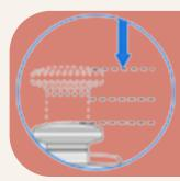
Dip the pipette tip into the liquid and slowly release to the original point.
