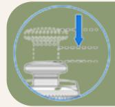
Before inserting the micropipette into the liquid, press the pump down to the first stopping point.
